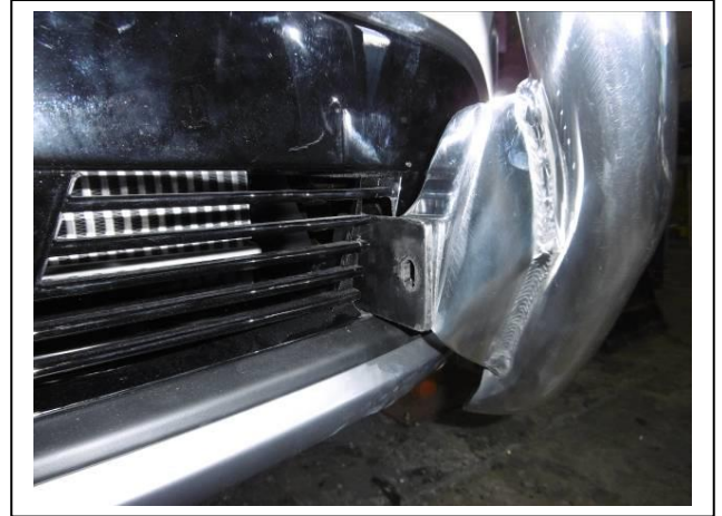
Figure 10: Fit protection bar onto steel mount.
