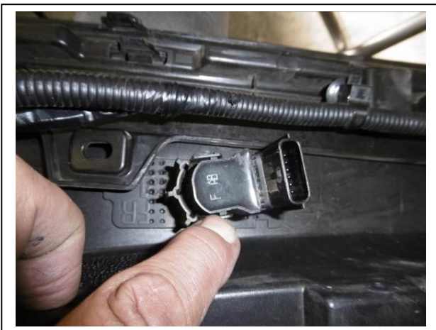
Figure 7: Remove inner sensors from bumper.
