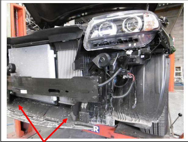
Figure 3: Remove lower half of air dams
