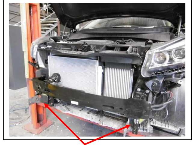
Figure 4: Steel mount fitted.
