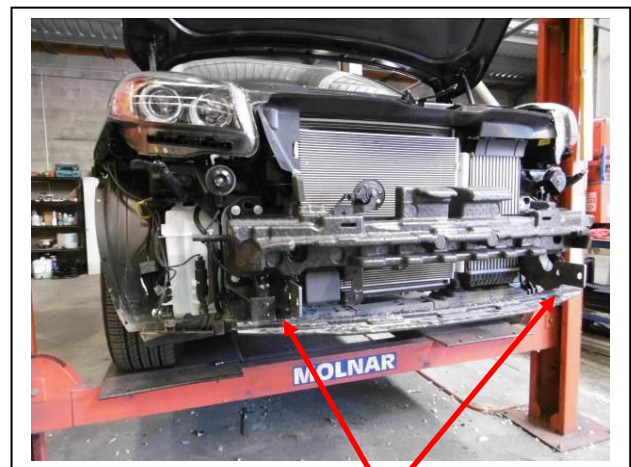
Figure 2: Remove lower bumper support, two 10mm bolts per side.
